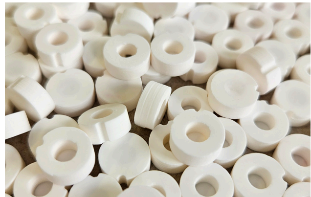
Additive Screen Printing is suitable for mass manufacturing in the millions, unlike most other additive manufacturing technologies. Image: ceramic sensors.
