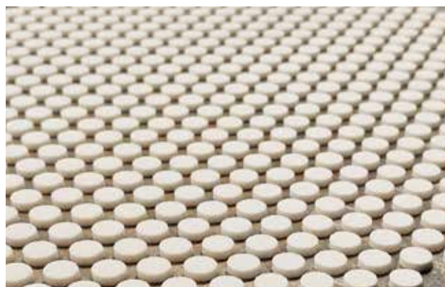
Additive screen printing enables the incorporation of multiple active pharmaceutical ingredients into tablets
