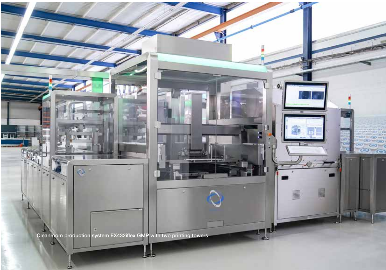
The gentle cold-printing technology enables the processing of active pharmaceutical ingredients
