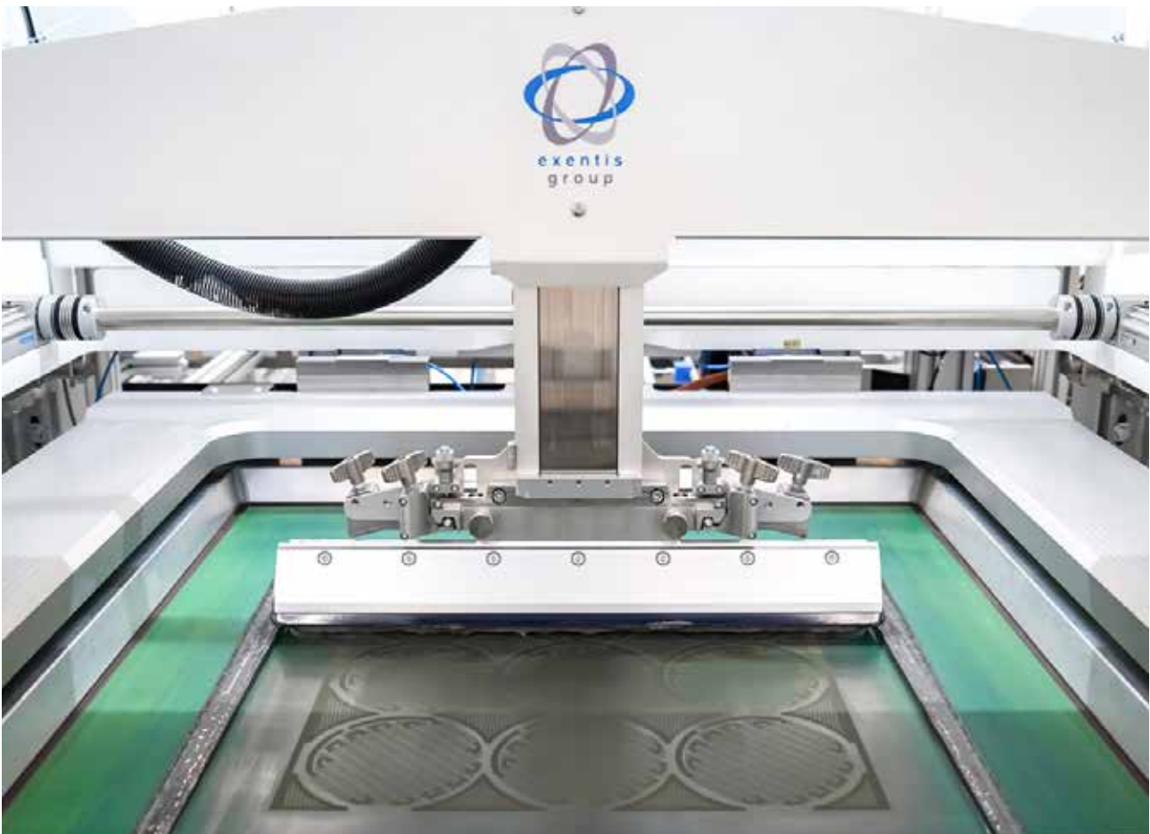
Printing heating elements on production system EX432i
